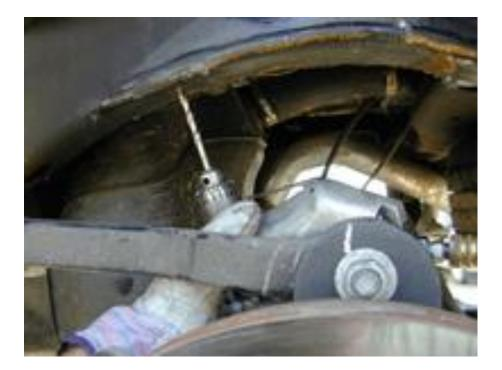
Jack the rear end back into place to make sure the new urethane button bump stop will align properly then drill and tap a  $3/8 \times 16$  threaded hole.
