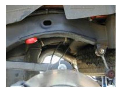
This is the frame after a little clean up with the grinder. Spending a little extra time all evidence of the bracket can be removed. Now you can see the very standard frame that was covered by the bracket.
