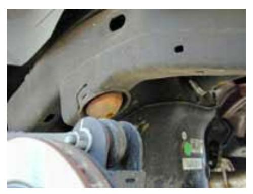
This is the stock bracket with the bump stop shortened. The ride was fair but can be greatly improved by completely removing the bracket from the frame.
