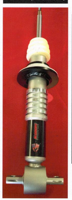
This strut in the box is set-up for a 1/2" drop.
