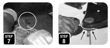
the spindle does not hit the control arm. If the spindle hits the control arm, remove the spindle and clearance the control arm more. <u>NOTE: WHEN THE BOLT GOES THROUGH THE</u> <u>SPINDLE IT, MUST ALSO GO THROUGH THE BALL JOINT</u> <u>RETAINING GROOVE INORDER TO LOCK IN PLACE.</u>
